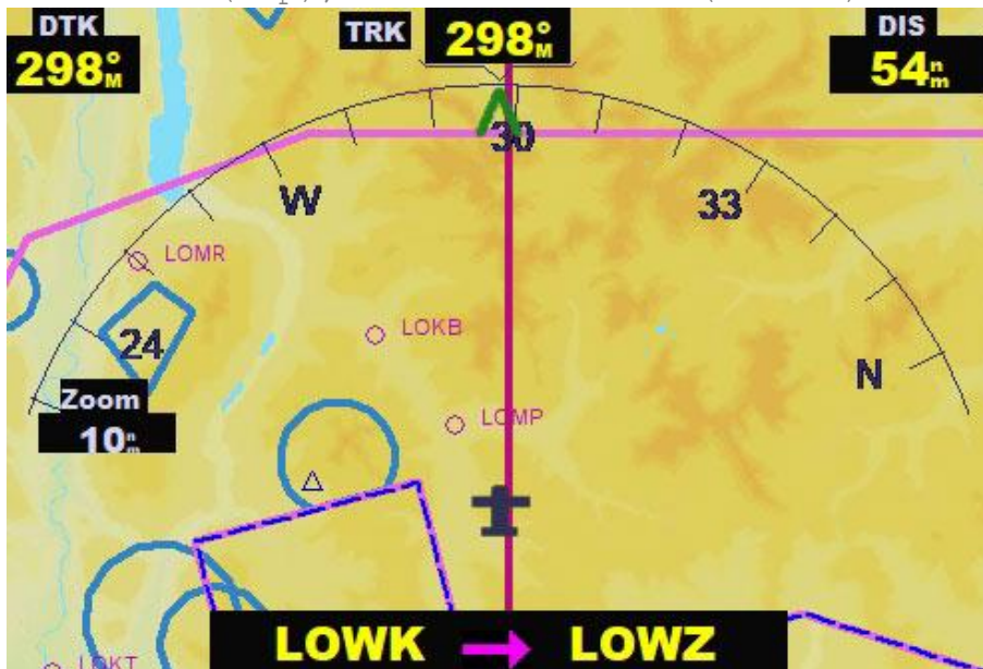
Only minimally visible deviation at zoom 10nm, nevertheless air traffic control will complain. Recommendation: Set the GPS zoom to 1-2nm.
